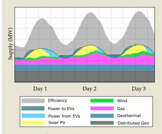
**Dynamics of a low-carbon system:** The integrated model provides an hourly examination of how the elements of NGU work together to meet demand. This 3-day summer supply profile illustrates the effects of efficiency, renewable energy, distributed generation, and storage from electric vehicles.
