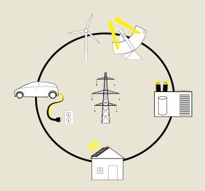
**Next Generation Utility:** The NGU system is based on five elements: energy efficiency, renewable energy, distributed generation, demand response, and energy storage, especially from electric vehicles.
